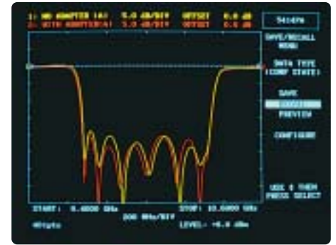
The Return Loss measurements (above) were created by the same bandpass filter. Measurement was performed with and without a test port adapter. Differences in the ripple display are caused by the vector error signal of the adapter's SWR reflection, which alternately adds and subtracts from the true return loss magnitude.
