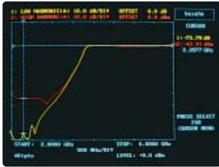
Errors due to source harmonics are most evident when testing wide band filters. As the source's fundamental frequency passes 2 GHz, the -33 dBc second harmonic is at 4 GHz – within the pass band of the wideband filter.
